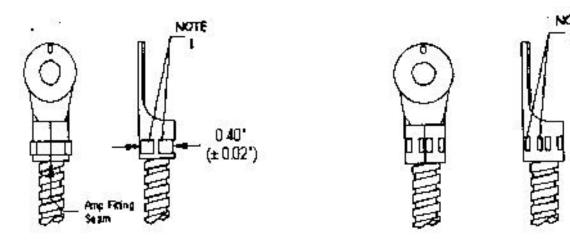
Inspection may require removal of the shrink-wrap. Incorrectly swaged fittings need to be repaired immediately. Copies of SB#091098 are available from Relative Workshop.
