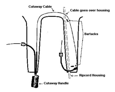
Soft housings can be replaced with metal housings by a qualified Rigger "A" as long as they only require hand tacking. Any required machine sewing would need to be performed by a Rigger "B". Details of housing change-over can be obtained from Sun Path Products Inc., 5037 Gall Blvd., Zephyrhills, Florida 33541 Phone: (813) 782-9242 Fax: (813) 788-3057
