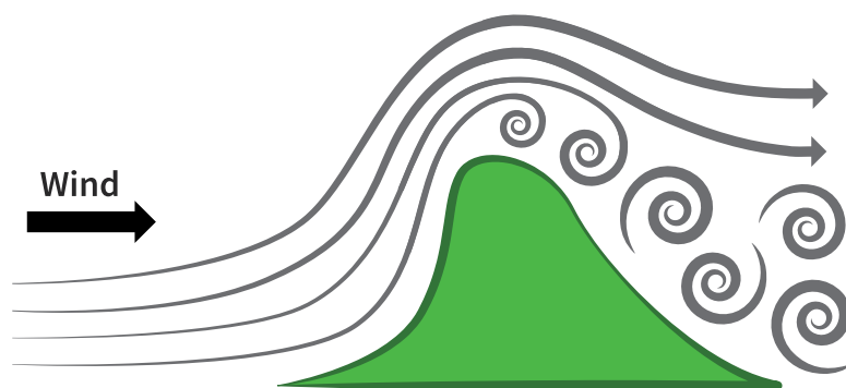
Figure 54: Turbulence Downwind of Obstacles
