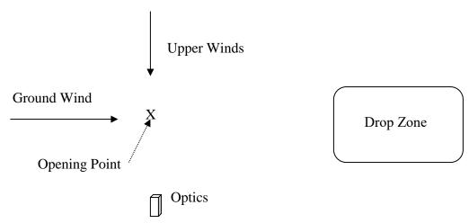
It should be noted that with a tail wind, the jumper will drift towards the optics while in freefall, whereas with a head wind the drift will be away from the optics. The former is better from an operational and evaluation viewpoint.
